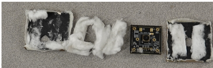
(c) Disassembled second-generation camera during the failure analysis.
