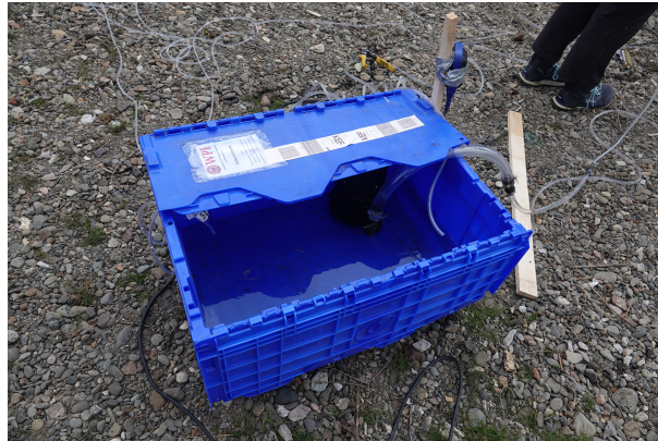
Figure 8: Cooling water reservoir and pump system
