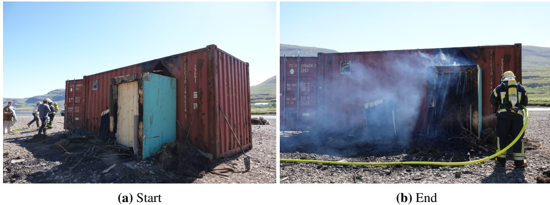
Figure 23: Photos of door scale Burn 6
