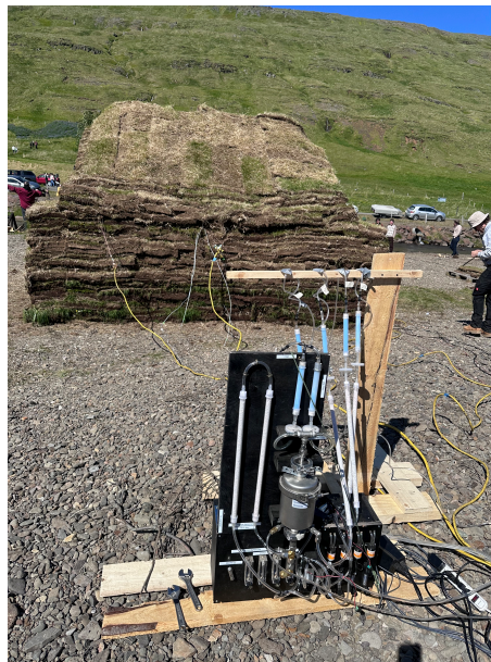
Figure 7: Gas sampling setup installed for the full scale test
