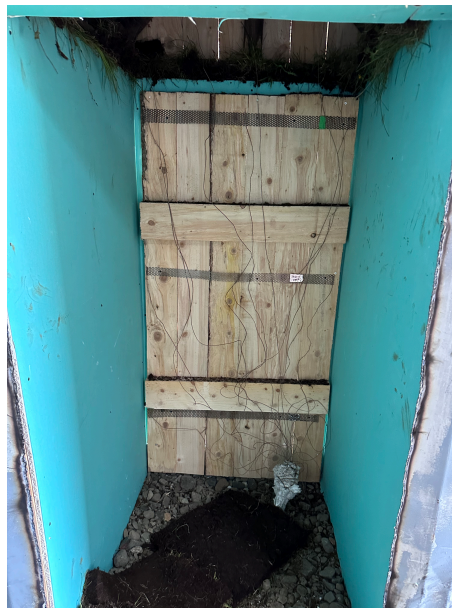
Figure 6: Thermocouples preassembled on metal meshes mounted to the door
