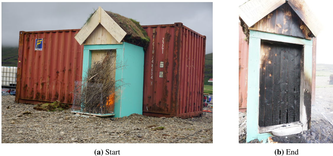
Figure 18: Photos of door scale Burn 1
