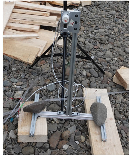
(b) Radiative heat flux gauge mounted on the stand
