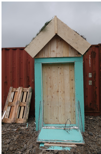
Figure 14: Door scale replica door and roof assembly attached to shipping container
