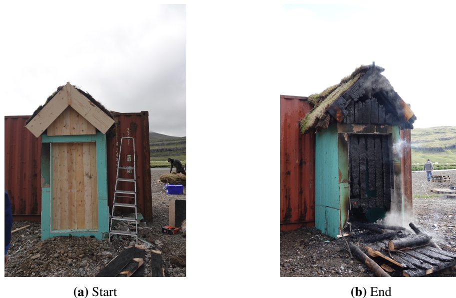
Figure 20: Photos of door scale Burn 3
