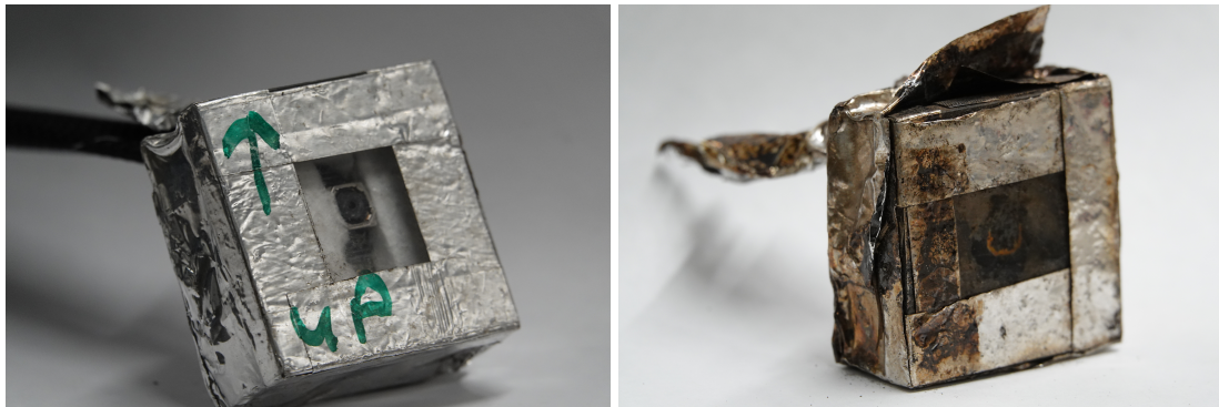
(a) Functioning second-generation camera used in the door-scale burns. (b) Second-generation camera after the full-scale burn.
