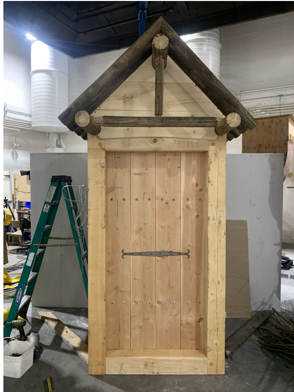
Figure 9: Lab scale door and roof assembly without turf
